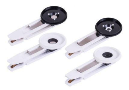
Continuous excitation fluorescence systems like Pocket PEA, Handy PEA+ and M-PEA rely on the use of a suitable leafclip system with 2 functions. Firstly, the leafclip shields the fluorescence detector from ambient light which would otherwise "blind" the sensor due to the comparatively high levels of red/infrared light within the same waveband as the fluorescence itself. Secondly, the leafclip pre-conditions or dark adapts a section of the sample prior to the measurement.
